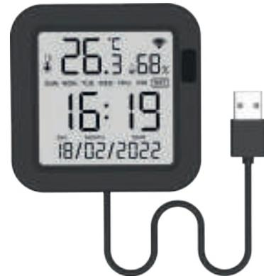
**CONTROL REMOTO IR UNIVERSAL CON SENSOR TEMPERATURA Y HUMEDAD**
